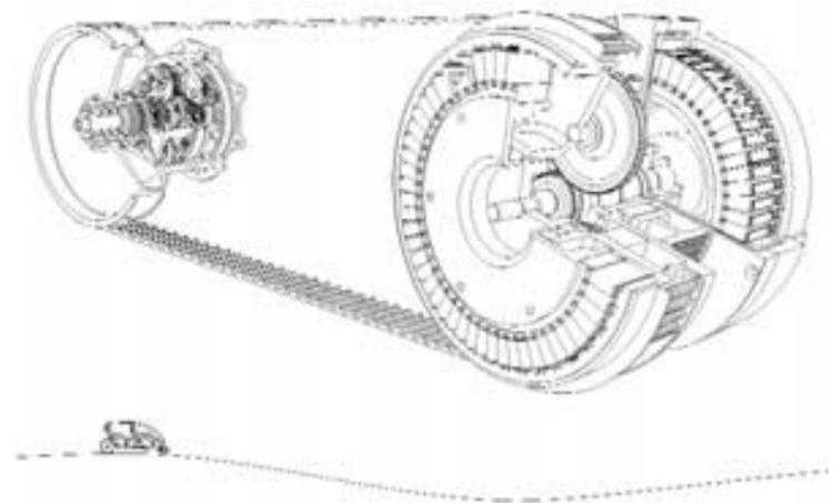
The Läufer's electric-assist transmission uses motor/generators on the intermediate driveshaft to 'even out' the gaps between the Rohloff's gears
